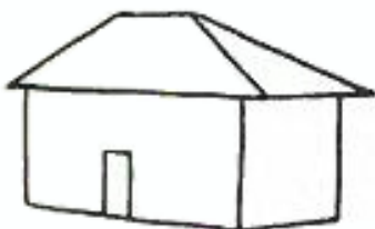
Diagram of Hipped roof
