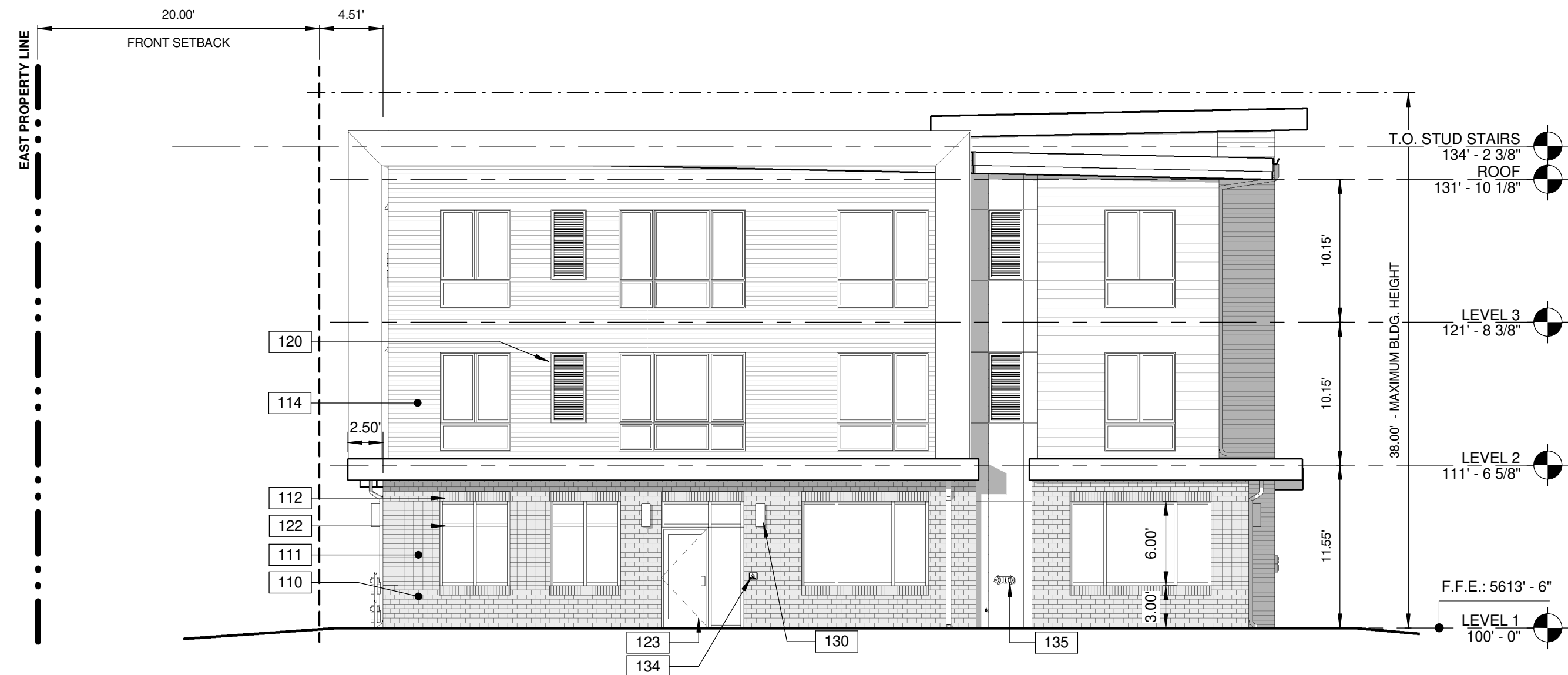
2 NORTH (DRIVE AISLE) EXTERIOR ELEVATION 1/8" = 1'-0"
