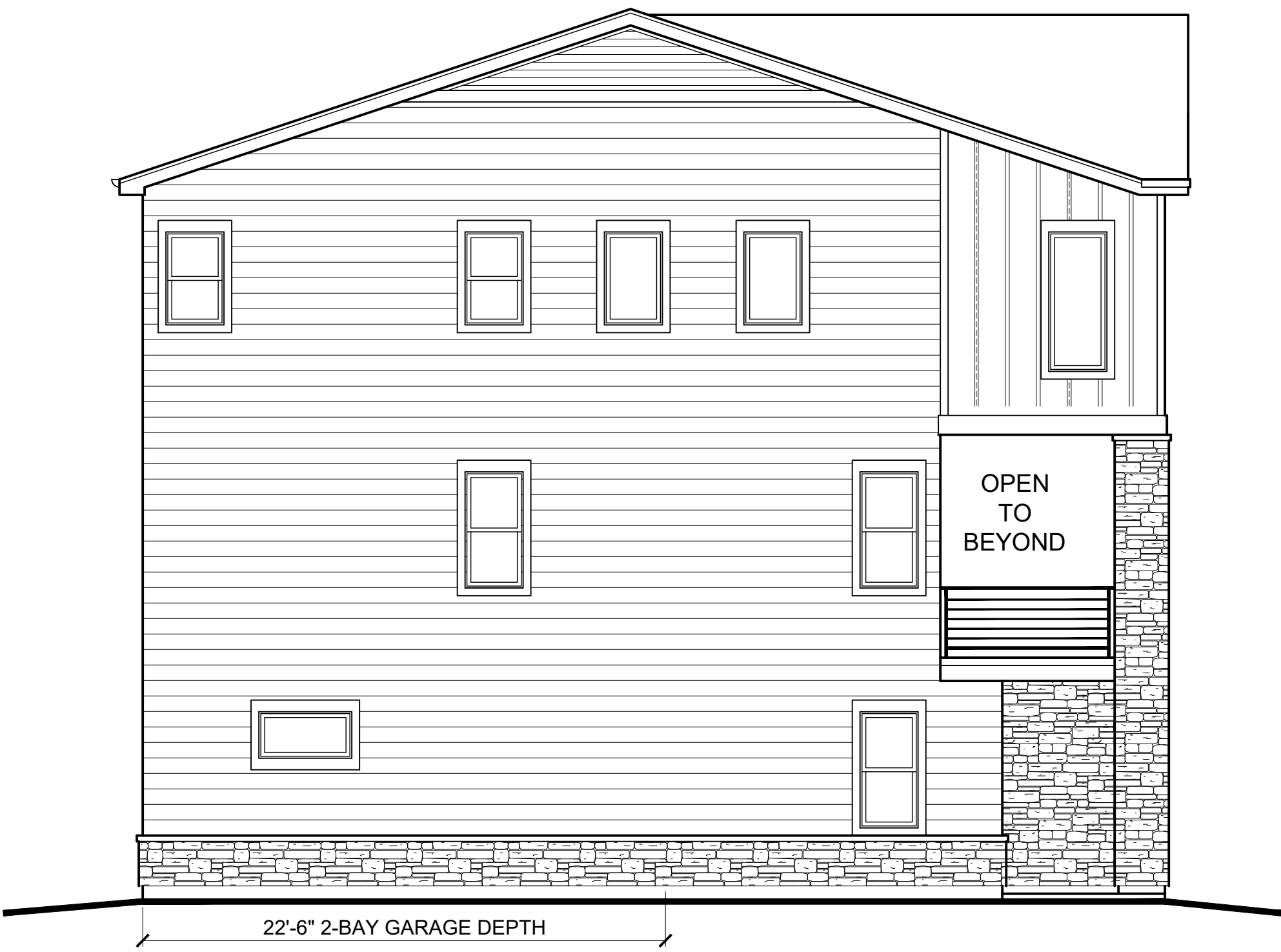
2 PLAN 3 LEFT ELEVATION - 'A' 15% MASONRY SCALE: 3/16" = 1'-0"
