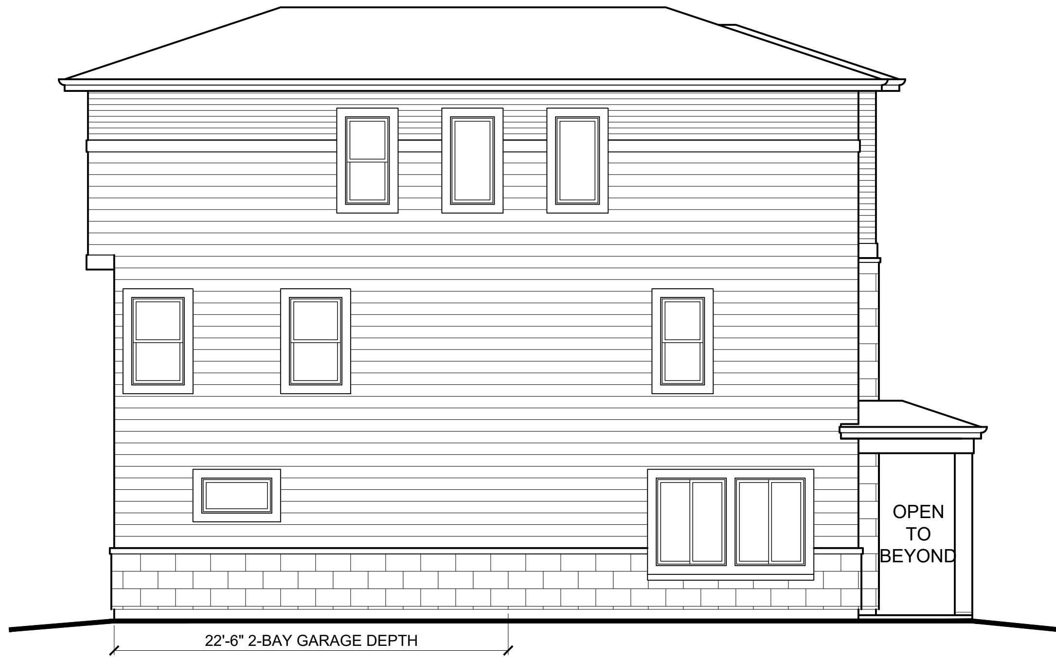
2 PLAN 4 LEFT ELEVATION - 'C' 12% MASONRY SCALE: 3/16" = 1'-0"
