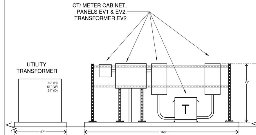
**C** EVSE EQUIPMENT ELEVATION DETAIL
