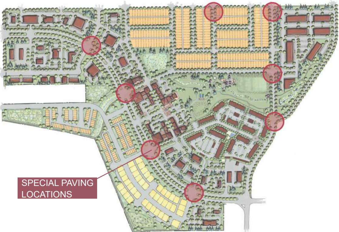
Special Paving Design Map - shows locations where special paving design will occur within Aurora One
