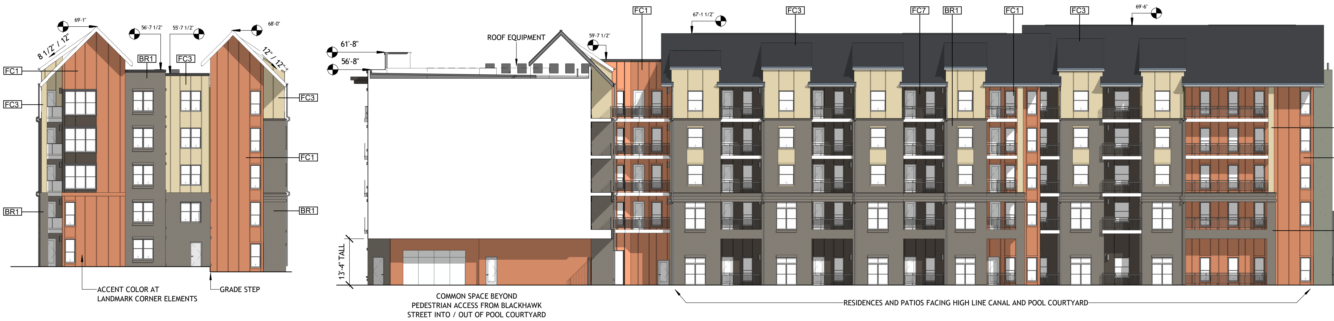
3 ELEVATION - EXTERIOR - B300 - SOUTH (LEFT) SDP XA3.02 1/16" = 1'-0" BRICK SF: 3,545 FIBER CEMENT SF: 2,402
