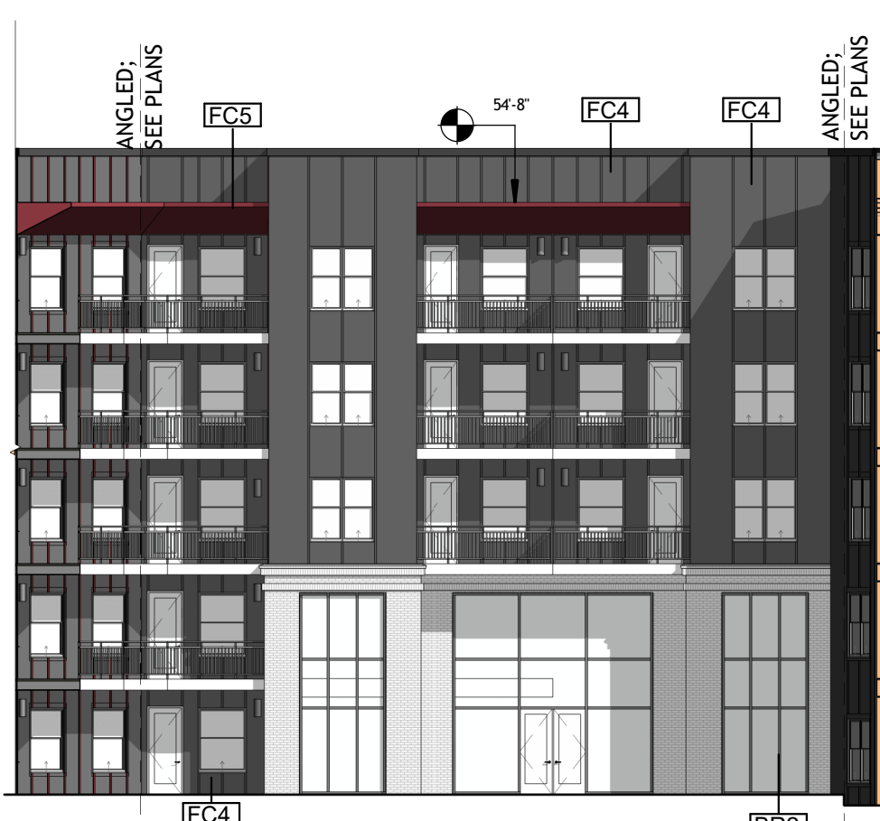
3 ELEVATION - EXTERIOR - B500 - PRIVATE COURTYARD - (WEST/LEFT) SDP BRICK SF: 928 FIBER CEMENT SF: 1,932 XA3.22 1/16" = 1'-0"
