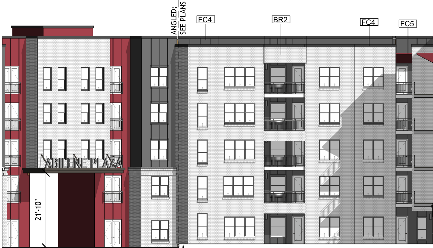
1 ELEVATION - EXTERIOR - B500 - PRIVATE COURTYARD (SOUTH) BRICK SF: 2,661 FIBER CEMENT SF: 1,342 XA3.22 1/16" = 1'-0"
