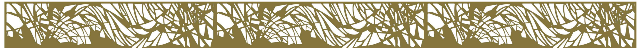
PATTERNED CUT STEEL PANELS (3/8" THICK STEEL, PAINTED OR POWDER COATED)
