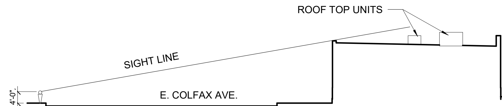
3 BUILDING A - E. COLFAX AVE. RTU VIEW SDP
