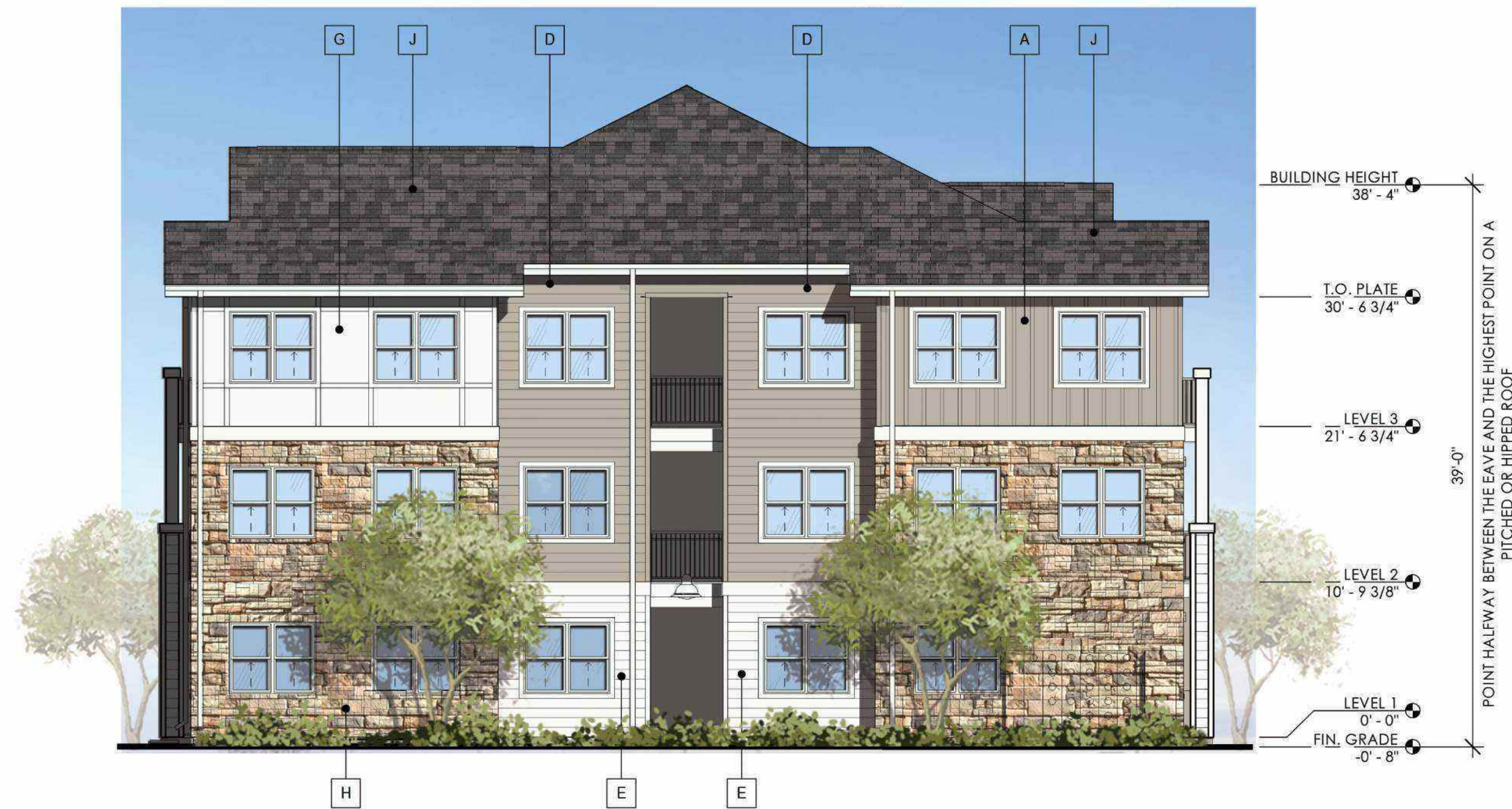
2 BUILDING TYPE 1 - LEFT ELEVATION 1/8" = 1'-0"
