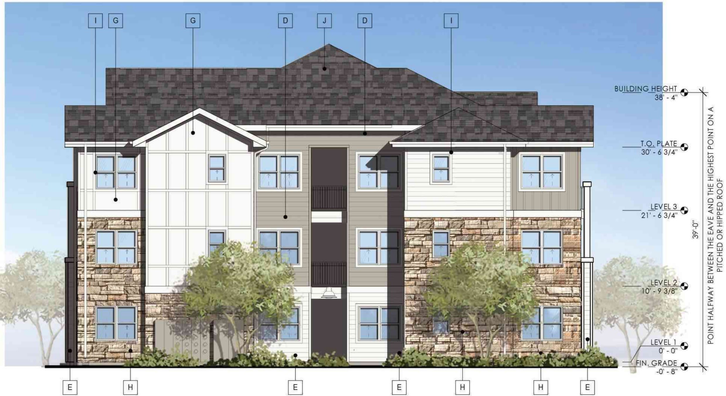
1 BUILDING TYPE 4 - WEST ELEVATION 1/8" = 1'-0"
