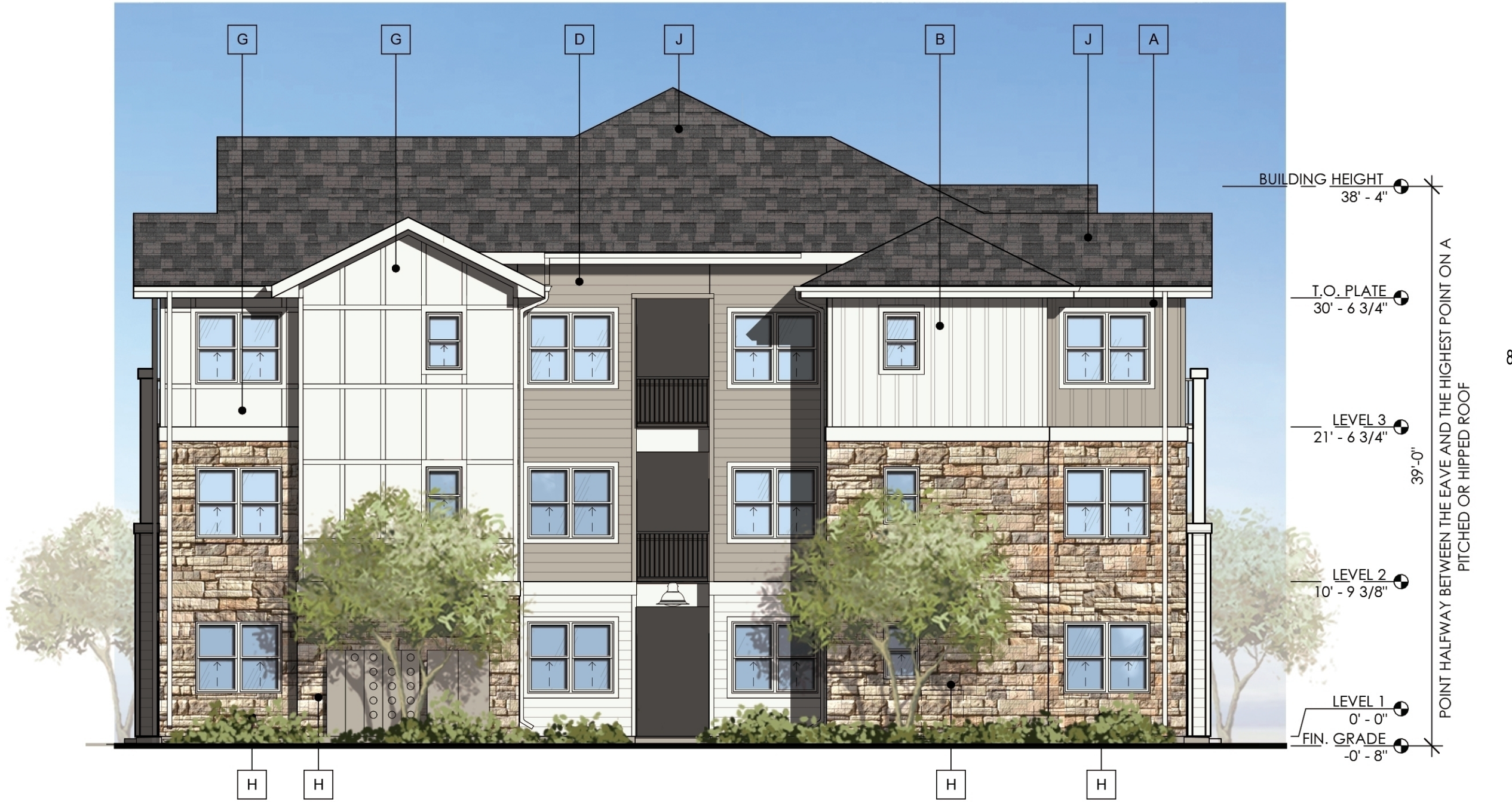
2 BUILDING TYPE 3 - RIGHT ELEVATION 1/8" = 1'-0"
