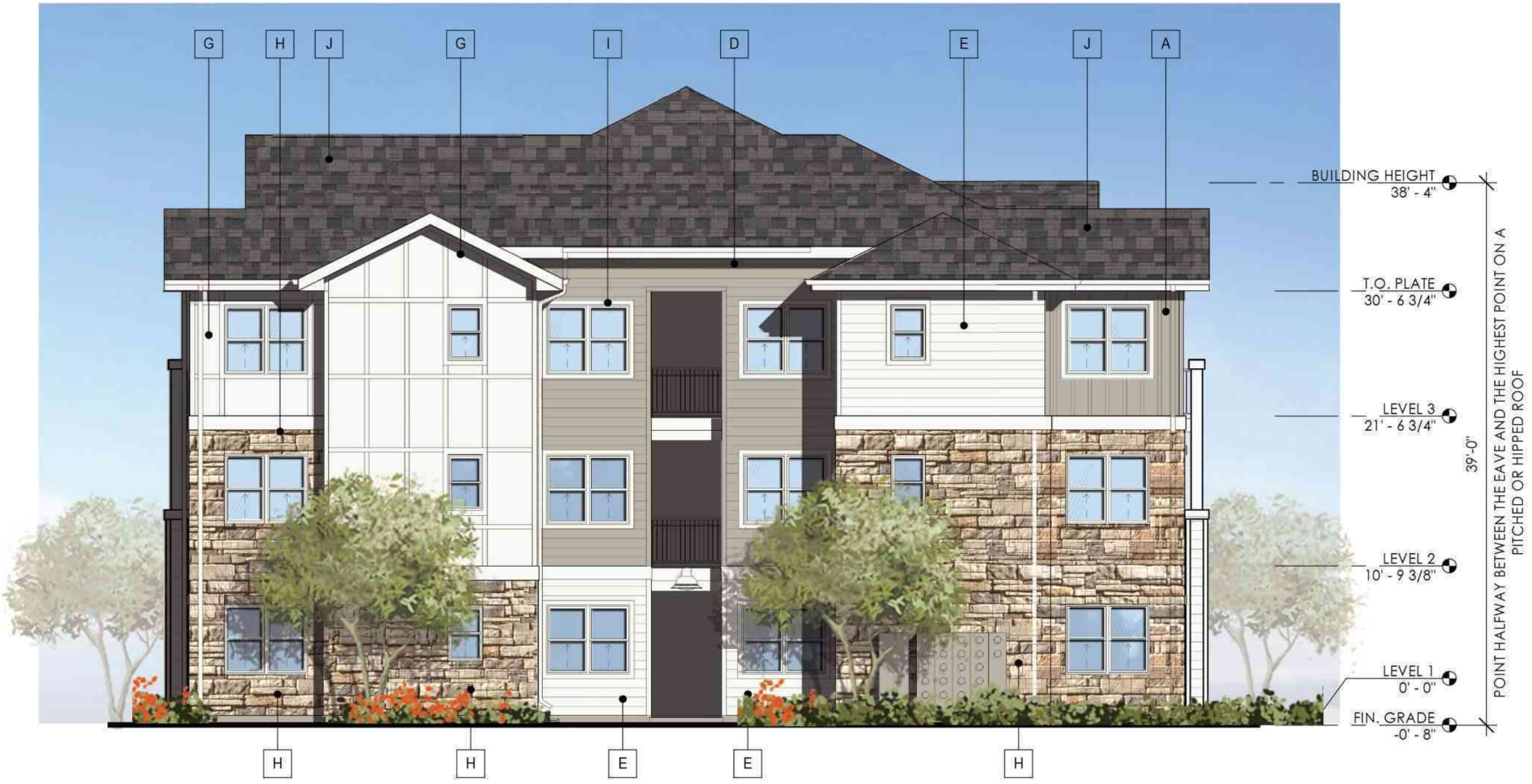
1 BUILDING TYPE 4 - WEST ELEVATION 1/8" = 1'-0"
