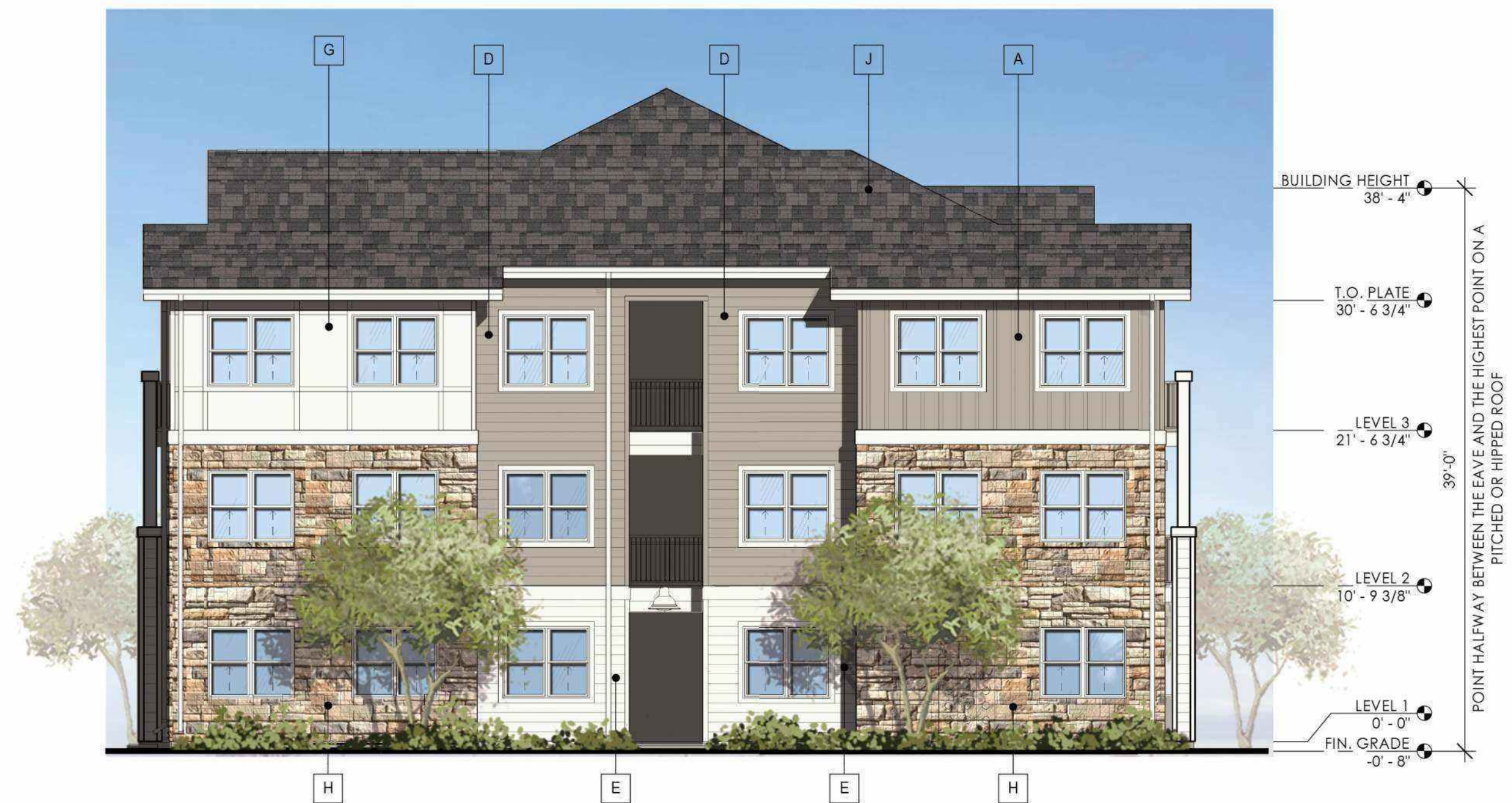
2 BUILDING TYPE 2 - LEFT ELEVATION 1/8" = 1'-0"
