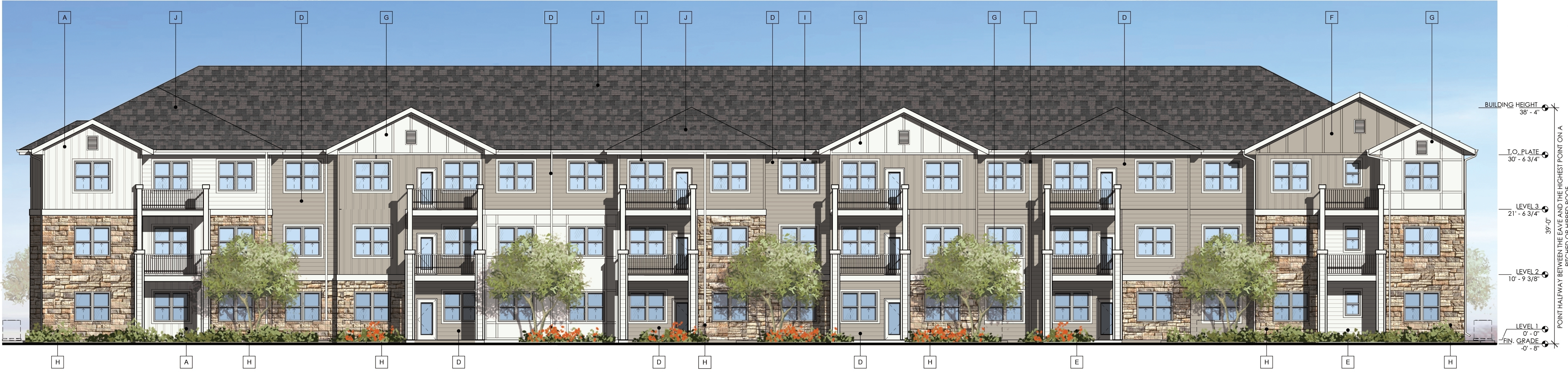
1 BUILDING TYPE 3 - REAR ELEVATION 1/8" = 1'-0"
