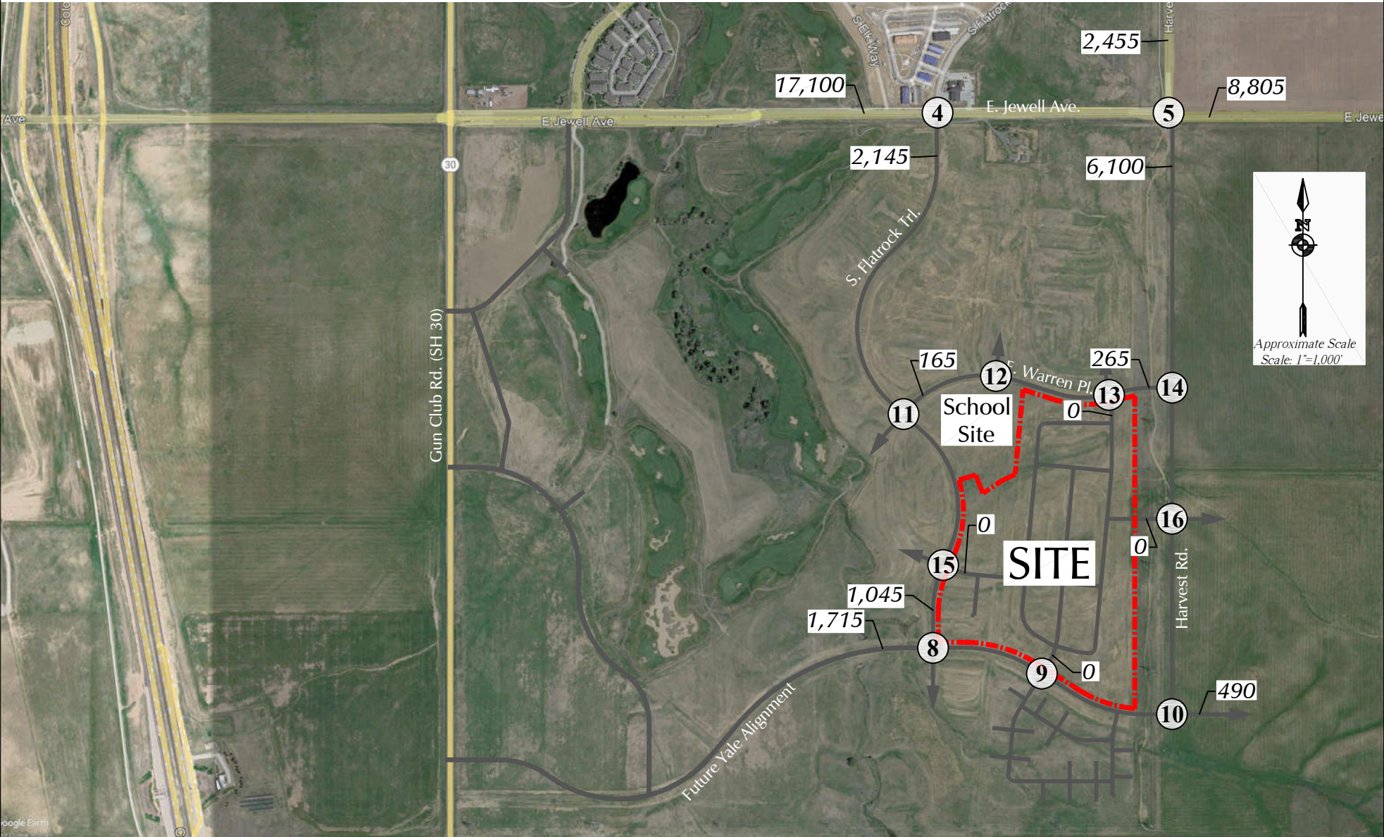
LEGEND: = Stop Sign = Traffic Signal \frac{26}{35} = AM Peak Hour Traffic \frac{35}{26} = PM Peak Hour Traffic 1 000 = Average Daily Traffic Yale & Jewell Intersections - Year 2024 Background Traffic, Lane Geometry and Traffic Control Murphy Creek East Filing 3 (LSC #220660) Figure 4a
