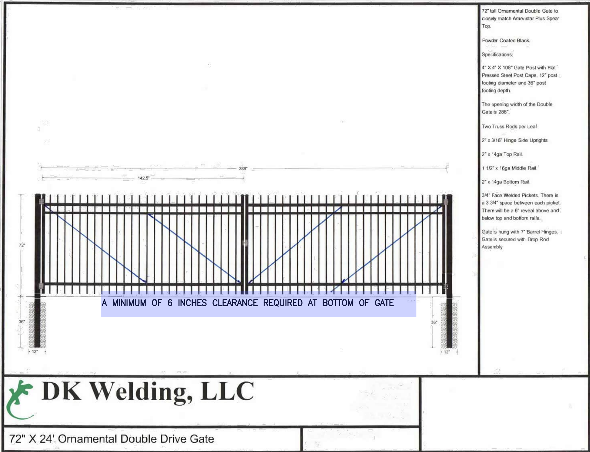
DETAIL 2: 24' SWINGING DOUBLE GATE
