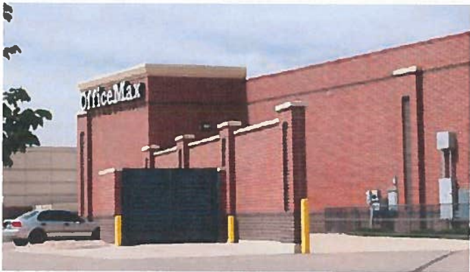
7E. Loading dock areas and trash receptacles screened from view and enclosed with materials matching main building
