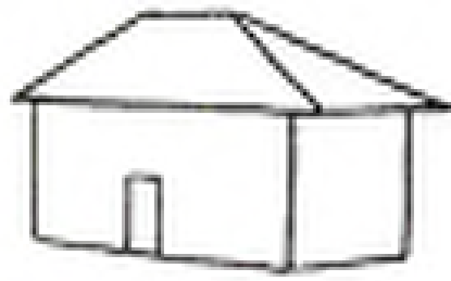
Diagram of Hipped roof
