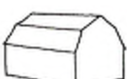
Diagram of Gambrel roof
