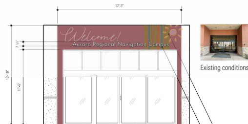
A1 EXTERIOR ELEVATION @ MAIN ENTRY DOORS 1/4" = 1'-0" Sign EE100 Entry Door Identification digitally printed exterior grade rough surface vinyl; clean surface as required prior to installation 1/2" thick flat cut out aluminum letters; mount with studs & silicone, as required; facility name only
