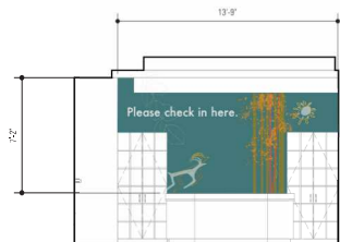
A3 INTERIOR ELEVATION @ CHECK-IN DESK 1/4" = 1'-0" Sign F103 Wall/Door Graphic digitally printed self-adhesive vinyl extend from ceiling to align with top of counter, wall-to-wall
