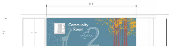
B4 INTERIOR ELEVATION @ CORRIDOR ELEVATOR LOBBY TO COMMUNITY ROOM, TYP. 1/4" = 1'-0" Sign F107, F202, F302, F402, F502 & F602 Wall/Door Graphic digitally printed self-adhesive vinyl extend from ceiling to top of baseboard, wall-to-wall; wrap engaged column at center of room Sign F107 shall be 7'-0" wide, field verify
