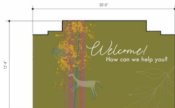
B2 INTERIOR ELEVATION @ COMMUNITY ROOM NORTH, TYP 1/4" = 1'-0" Sign F203, F303, F403, F503 & F603 Wall/Door Graphic digitally printed self-adhesive vinyl extend from ceiling to top of baseboard, wall-to-wall; wrap engaged column at center of room Sign F603 shall be divided into two, 5'-0" wide parts
