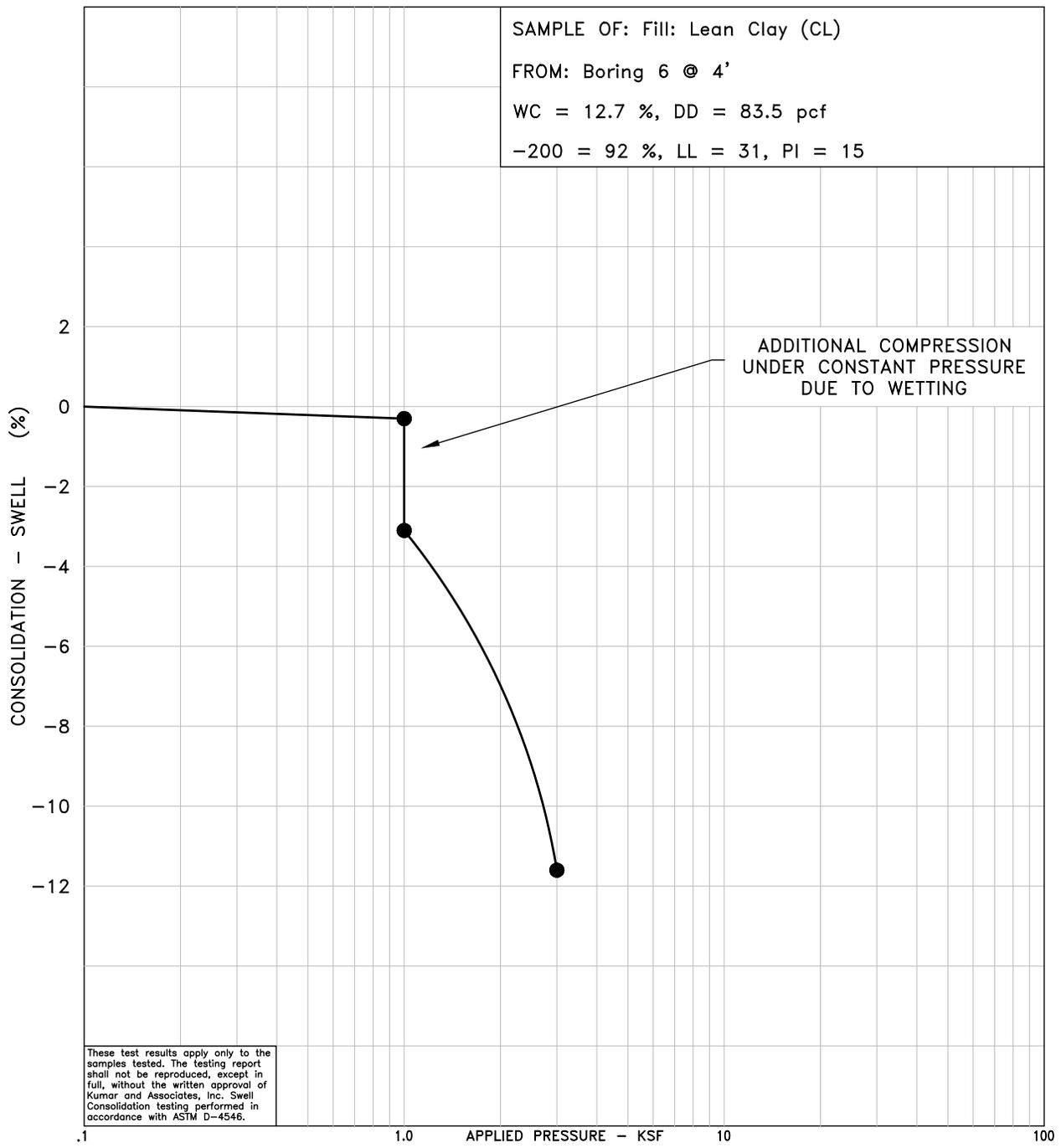
These test results apply only to the samples tested. The testing report shall not be reproduced, except in full, without the written approval of Kumar and Associates, Inc. Swell Consolidation testing performed in accordance with ASTM D-4546.
