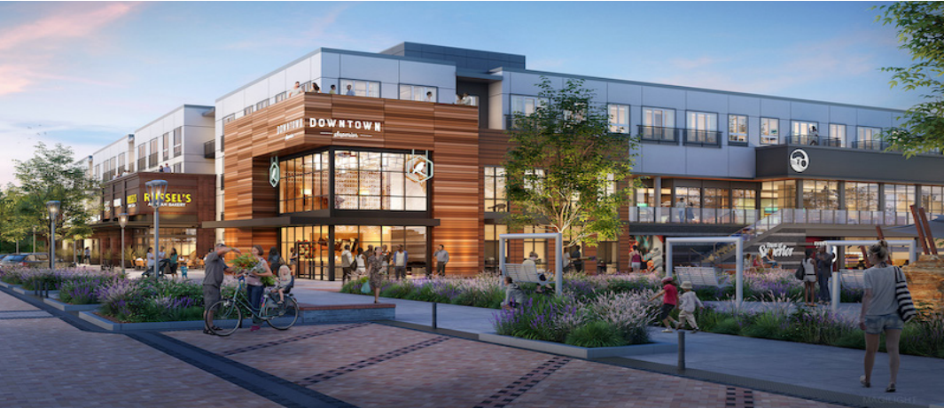
A Building using various projections and reveals to break down the scale of the building.
