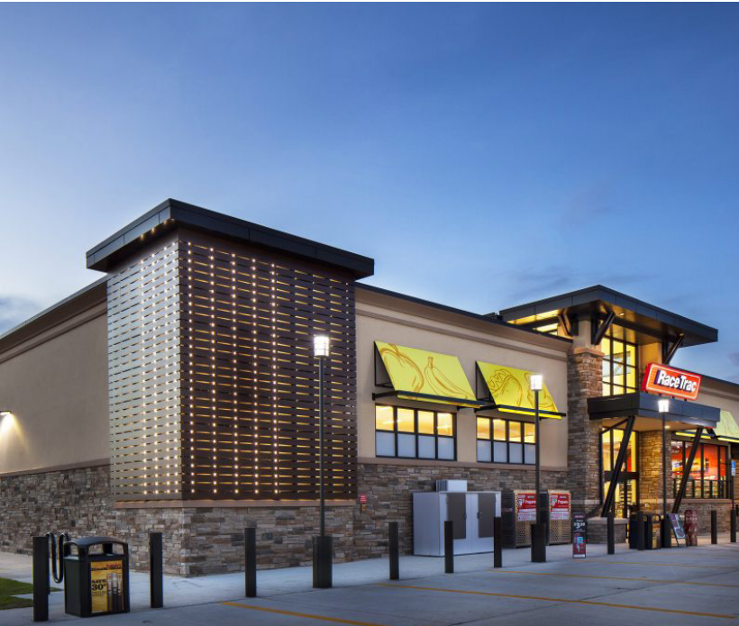
A parapet wall may be used to screen mechanical equipment.
