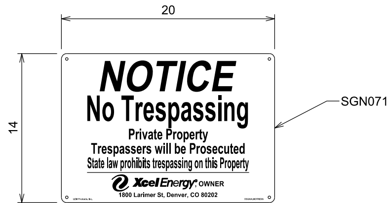
3 DETAIL - TYPICAL NO TRESPASSING SIGN (NT) NOT TO SCALE
