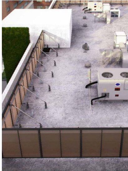
Figure 4.29: Rooftop mechanical equipment shall be screened from view from the street.
