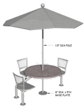
**NOTES:** ALL WELDED ALUMINUM CONSTRUCTION. TOP: 42" DIA. ROSETTE TABLE TOP WITH 2" DIA. UMBRELLA HOLE. BACK: WATERJET CUT TO MATCH PRESTON GRID. SEAT: DISHED ALUMINUM WITH SANDDOLLAR DRAIN HOLES. FABRY: SILVER SIDE - CLEAR COAT (ON ALL PARTS). GLIDE: BOLT-DOWN TABS. \*\*NO SWIVEL\*\*
