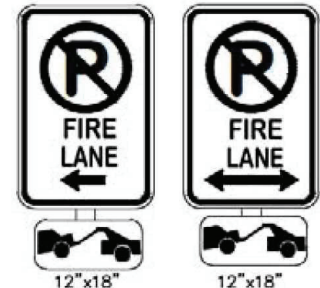
2 FIRE LANE PARKING SIGN DETAIL N.T.S.
